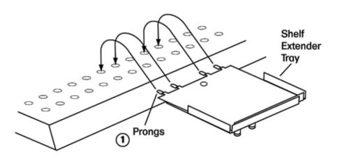
Pivot tray downward to secure tabs in shelf, so that tray aligns with shelf.
